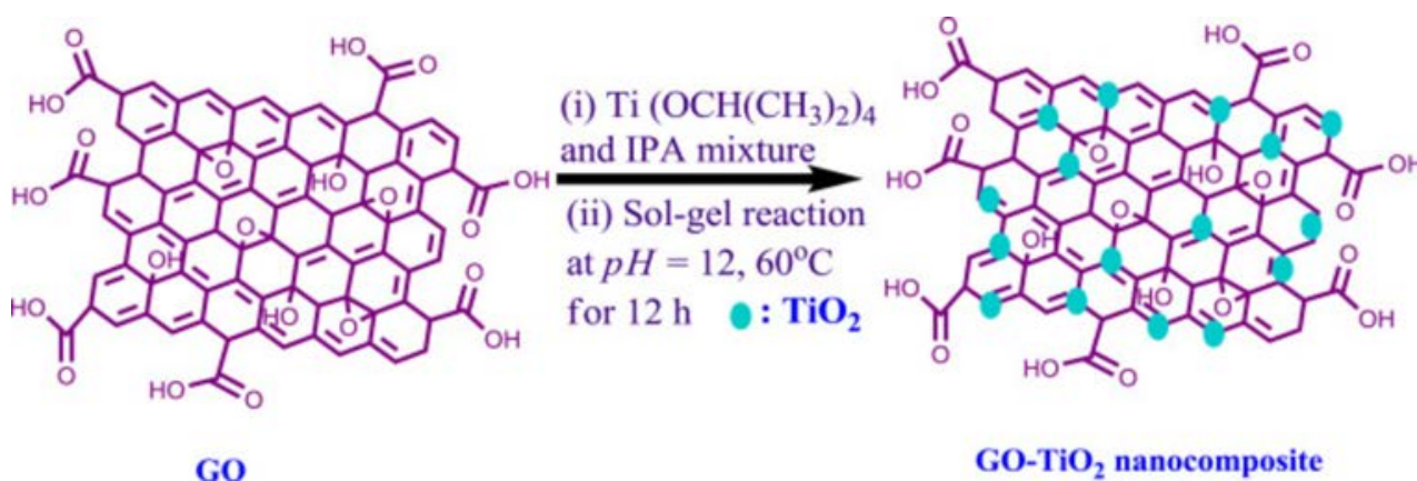
Figure 2.8. Schematic reaction route for synthesis of the GO–TiO 2 nanocomposite from GO nanosheets and TTIP via the sol–gel reaction at pH 2 and 60°C.
